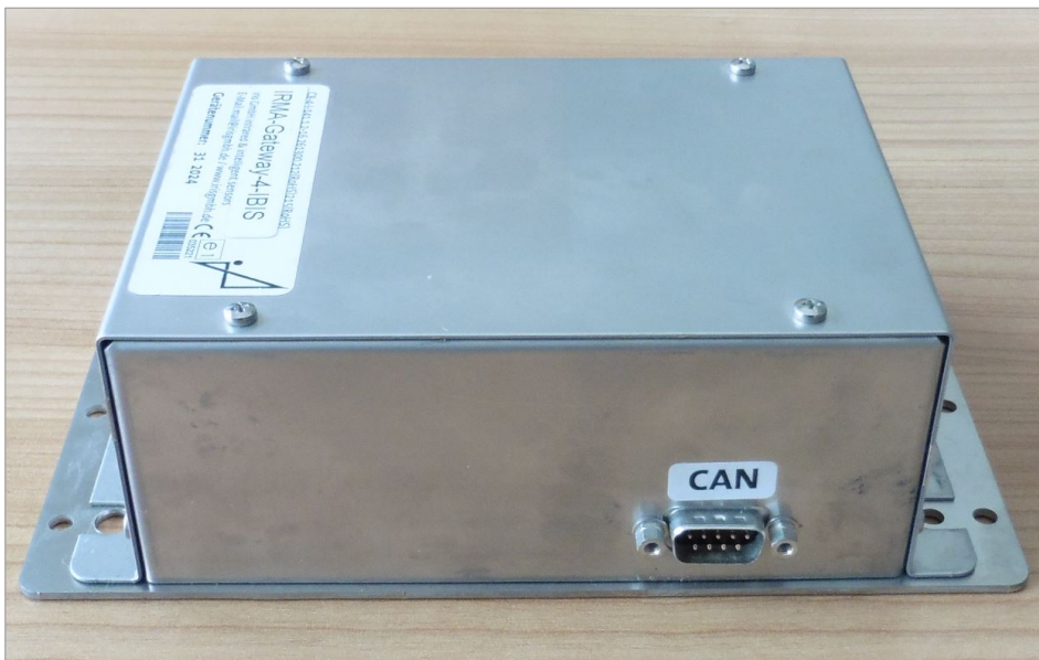
Fig. 3: View of IRMA-Gateway-4-IBIS sensor connector
