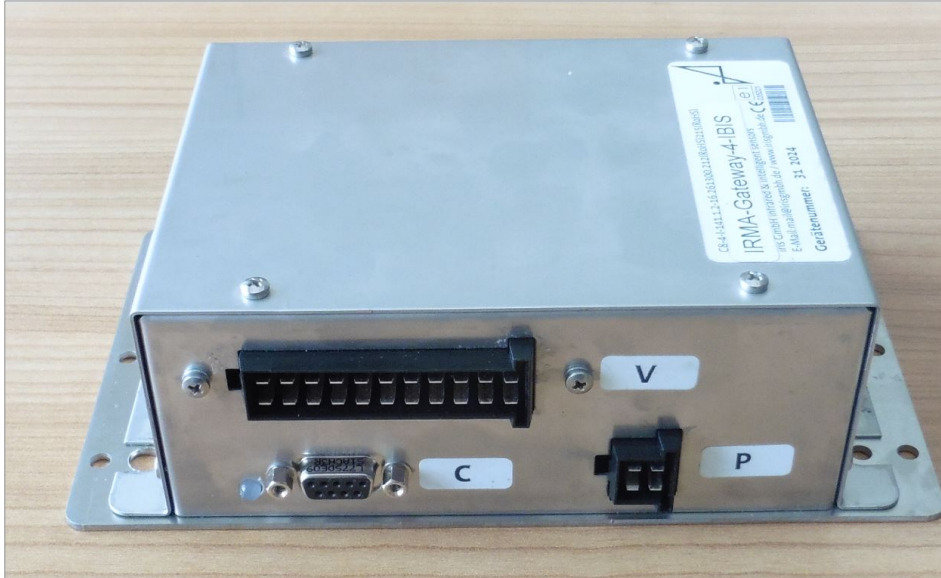
Fig. 2: View of IRMA-Gateway-4-IBIS interfaces and nameplate
